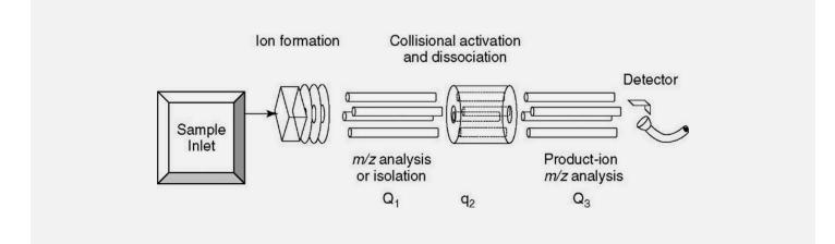
LC/MS/MS can optimize dwell times to improve sensitivity. During method development it's important to monitor multiple charge states to determine which will afford better selectivity and sensitivity. Also consider different ion pairing reagents to drive the charge envelope into the mass range of the instrument.
