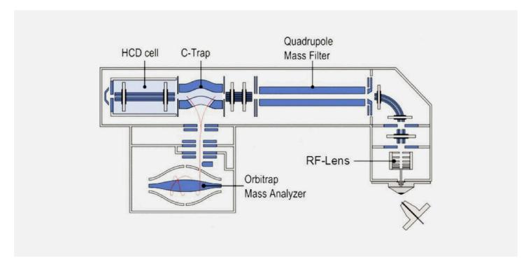
Two different data acquisition modes in LC/HRMS are TSIM (targeted selection ion monitoring) and Full Scan. TSIM will drop overall data points per monitored targeted mass points, and Full Scan offers data points for all masses and enables the ability to mine data post-acquisition. It's recommended to use TSIM when you need to identify specific compounds with high sensitivity and selectivity, and Full Scan when you're interested in identifying a wide range of compounds.
